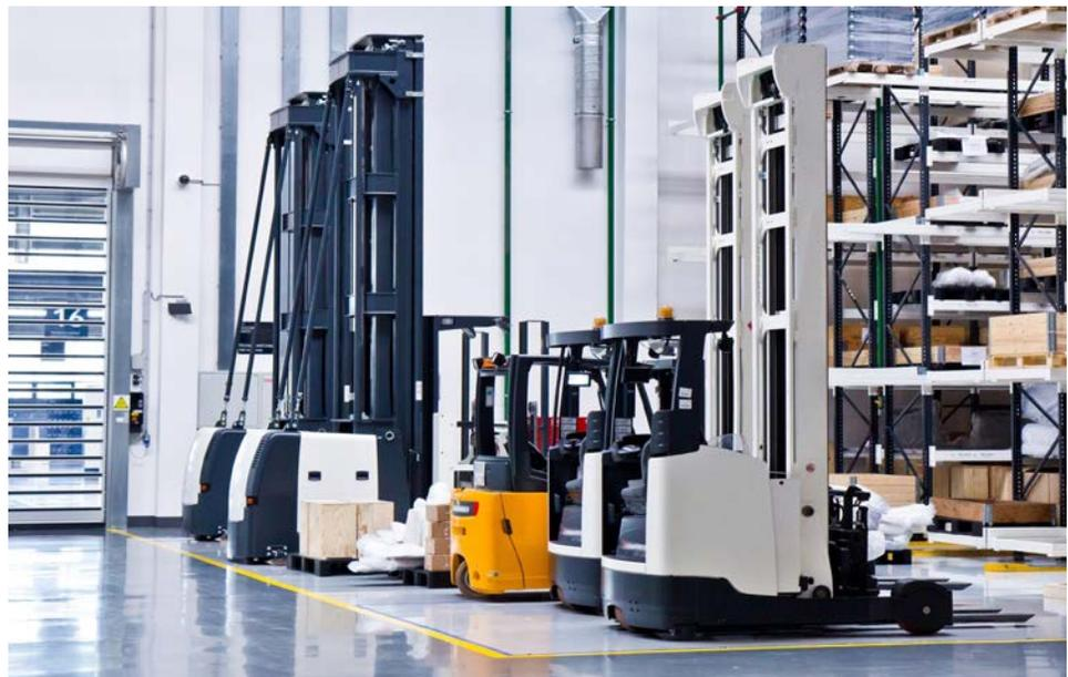
Driverless forklifts are nothing new, but their newfound freedom enabled by smart sensor technology certainly is. No longer limited to following a painted stripe on the floor, a new generation of autonomous forklifts use camera-based sensors to “see” an environment and make onboard decisions accordingly based on interpreted data. These forklifts can navigate complex routes from the loading dock to anywhere on the factory floor, while choosing the fastest and safest route.
